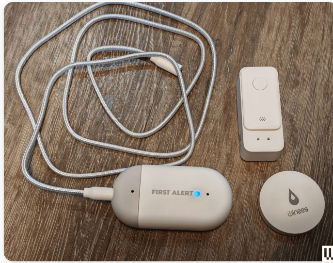
Figure 2) Water sensors catch the first drops under sinks and appliances.
